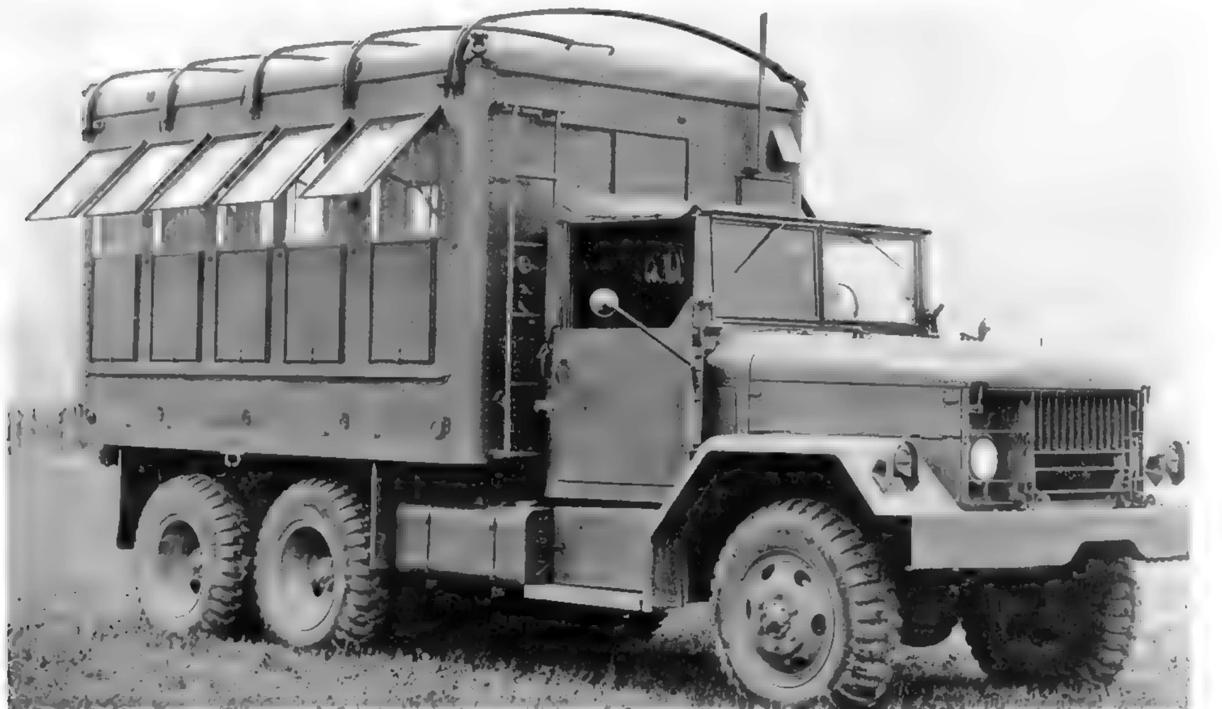
The M109 trucks also had provision for mounting bows, allowing canvas to be fitted to disguise the vehicle as a cargo truck. (National Archives and Records Administration photo)
